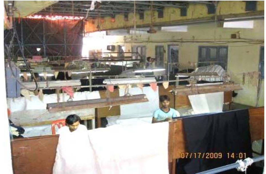
Workers spread cloth over lighted plates to spot defects
