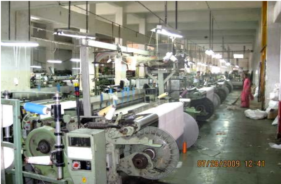
(3) Weaving the fabric on the weaving loom
