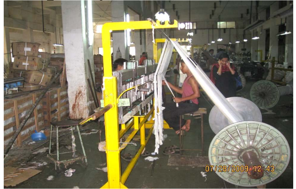
(2) Drawing the warp beam ready for weaving
